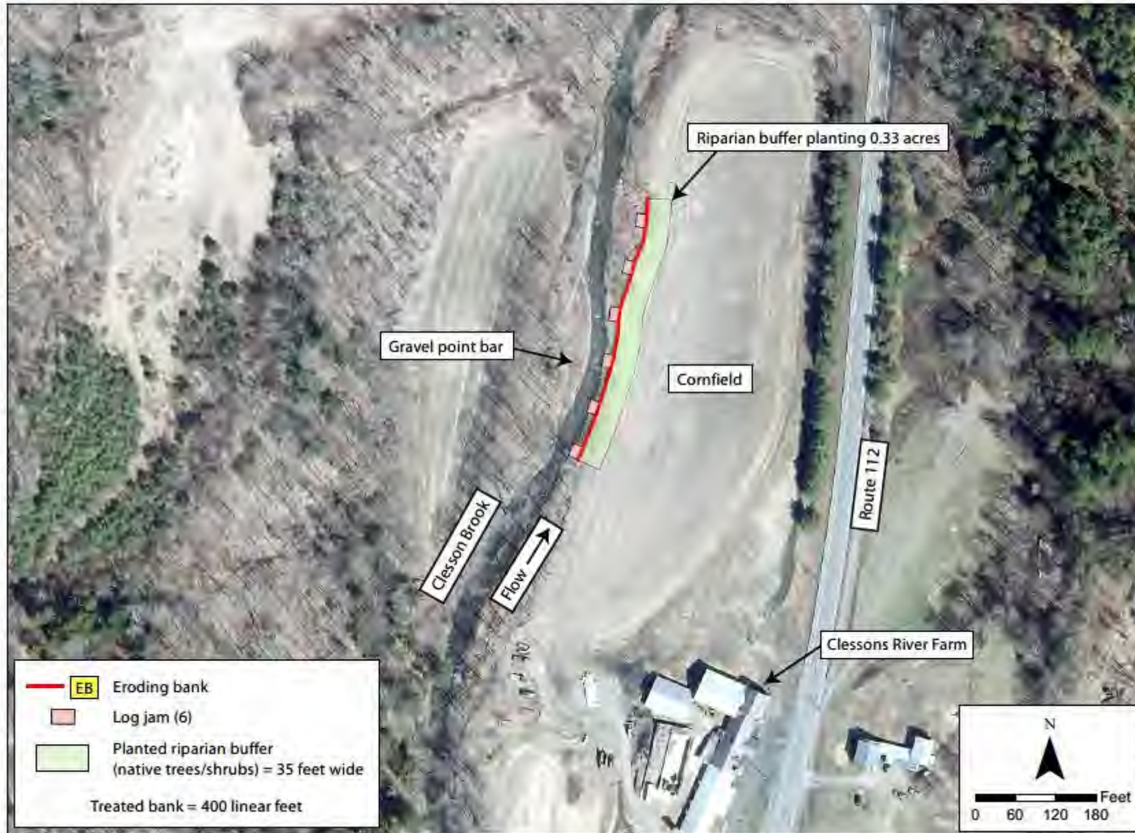
Clesson Brook - Clessons River Farm Site. Conceptual Design Plan View.
