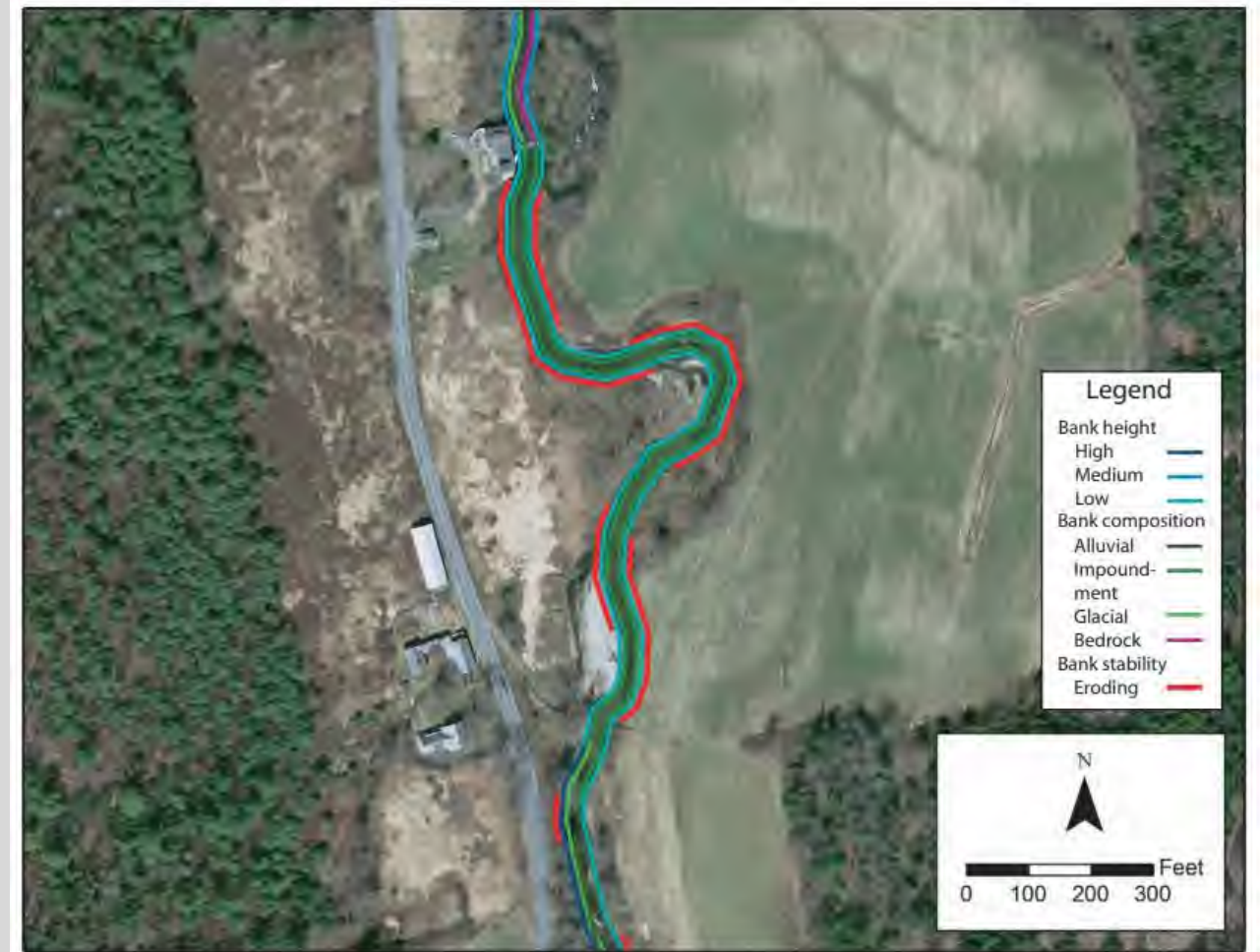
Figure 11. Comparison of bank composition (inner line), height (middle line), and stability (outer line) along a portion of South River.
